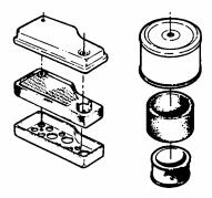
Generally, wash foam-type filters in a dishwashing detergent and water solution. Rinse and wring dry, then saturate with oil and squeeze out excess. Failure to re-oil this type filter will ruin the
